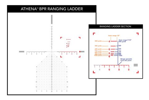
Horizontal ranging is calibrated for an 18" wide target. Simply line up the target's width with the appropriate line to determine range to target. For example, an 18" wide target that appears to be the same width as the ranging line with a "6" next to it will be 600 yards away. This method is useful when the target's height is partially obscured, as with a target in tall grass.
