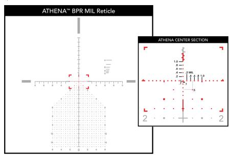
To the left and right of center, boxes are located at 0.2 MIL intervals with a slightly larger rectangle at 1.0 MIL from center for easy navigation. Small dots (0.05 MIL thick) are spaced at 0.2 MIL intervals above and below center for a total of 1.0 MIL distance. The first of the grid pattern dots are located 0.5 MIL down and left/right of center.
