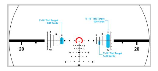
Because the crosshair runs halfway through each MIL stadia, you can also use the vertical stadia for ranging ~36" targets. This allows you to range crouched or partially concealed targets, holding crotch-to-head. For targets at extreme distances, you can use the half-stadia to range a target at double the indicated distance.
